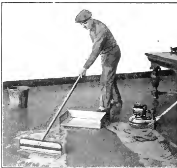
FIG. 4 THE SECOND STEP IS TO TAKE UP THE DIRTY WATER AFTER SCRUBBING WITH THE MACHINE IS FINISHED
